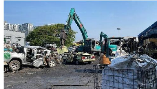
Dismantling Using Nibbler
